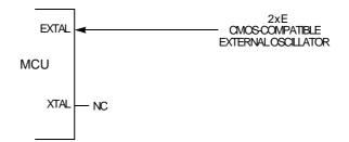
Figure 10 External Oscillator Connections
