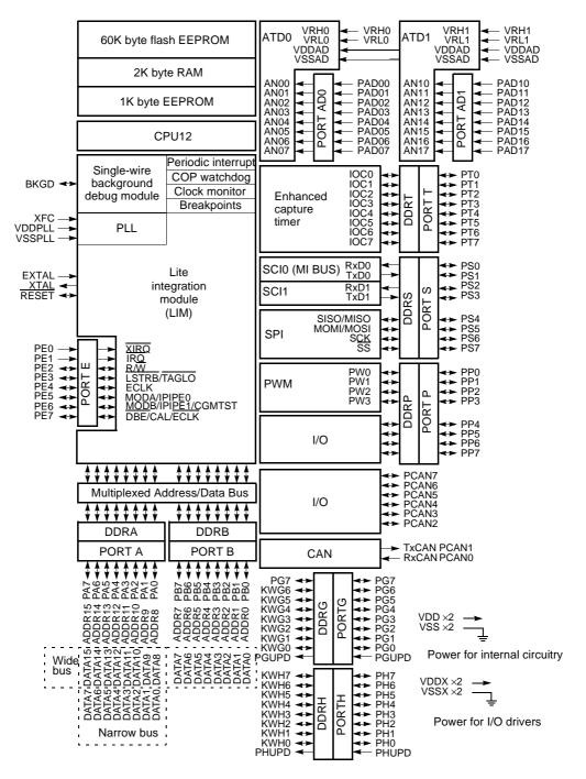
Figure 1 MC68HC912D60A 112-pin QFP Block Diagram
