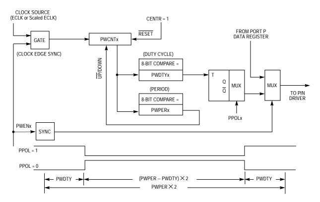
Figure 24 Block Diagram of PWM Center-Aligned Output Channel
