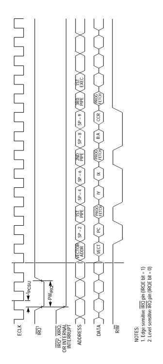
Figure 62 Interrupt Timing Diagram
