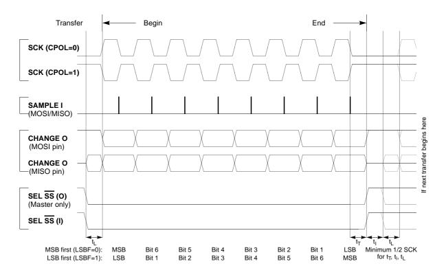
Figure 36 SPI Clock Format 1 (CPHA = 1)
