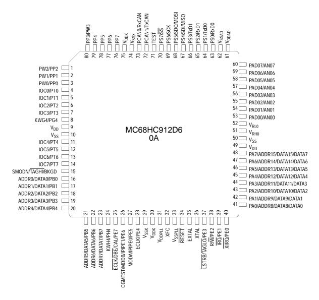
Note: TEST = On early production devices this pin is used for factory test purposes. It is recommended that this pin is not connected within the application, but it may be connected to VSS or 5.5V max without issue. On later production devices this pin is not bonded out.
