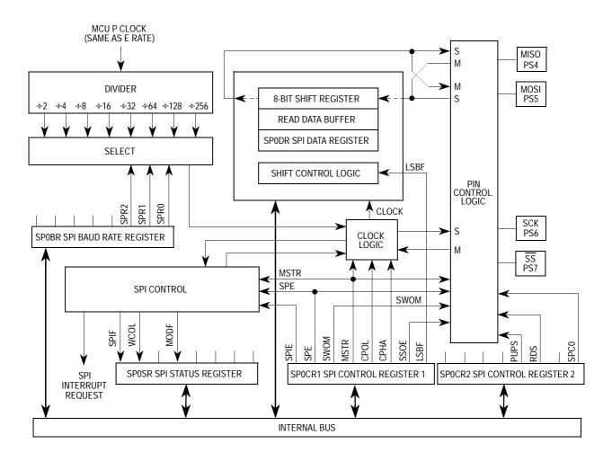
Figure 34 Serial Peripheral Interface Block Diagram
