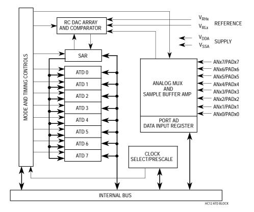
Figure 54 Analog-to-Digital Converter Block Diagram
