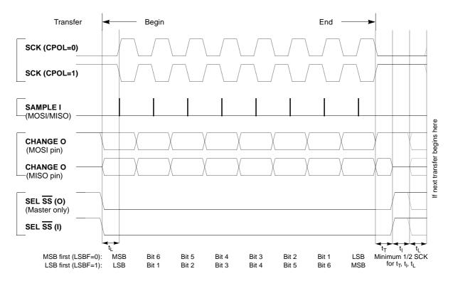
Figure 35 SPI Clock Format 0 (CPHA = 0)
