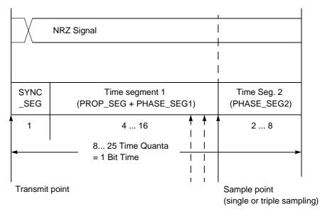
Figure 49 Segments within the Bit Time
