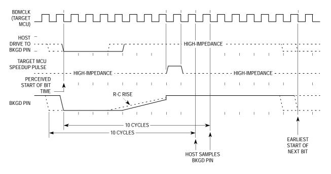
Figure 56 BDM Target to Host Serial Bit Timing (Logic 1)
