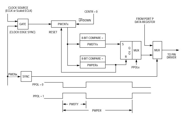
Figure 23 Block Diagram of PWM Left-Aligned Output Channel
