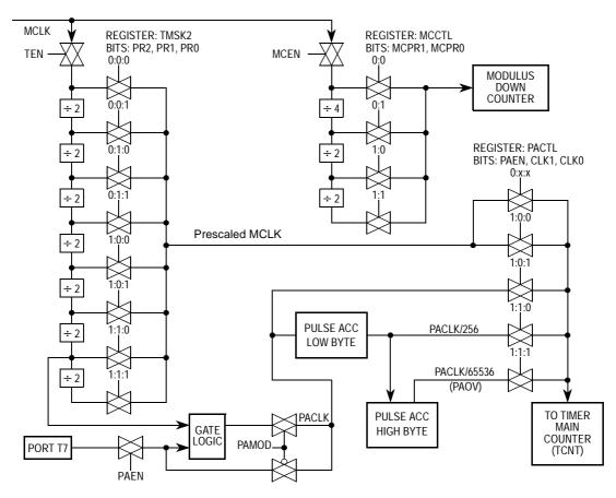
Figure 21 Clock Chain for ECT
