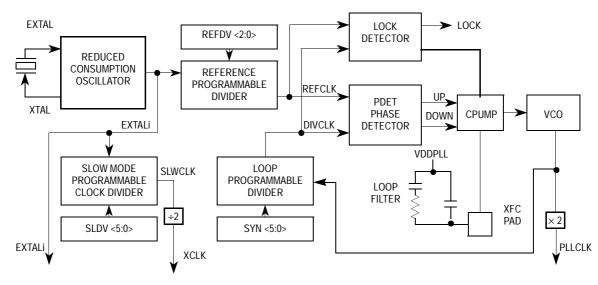
Figure 15 PLL Functional Diagram
