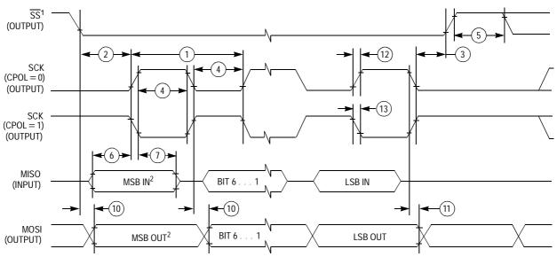
1.  $\overline{SS}$  output mode (DDS7 = 1, SSOE = 1). 2. LSBF = 0. For LSBF = 1, bit order is LSB, bit 1, ..., bit 6, MSB.
