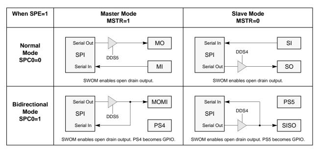
Figure 37 Normal Mode and Bidirectional Mode
