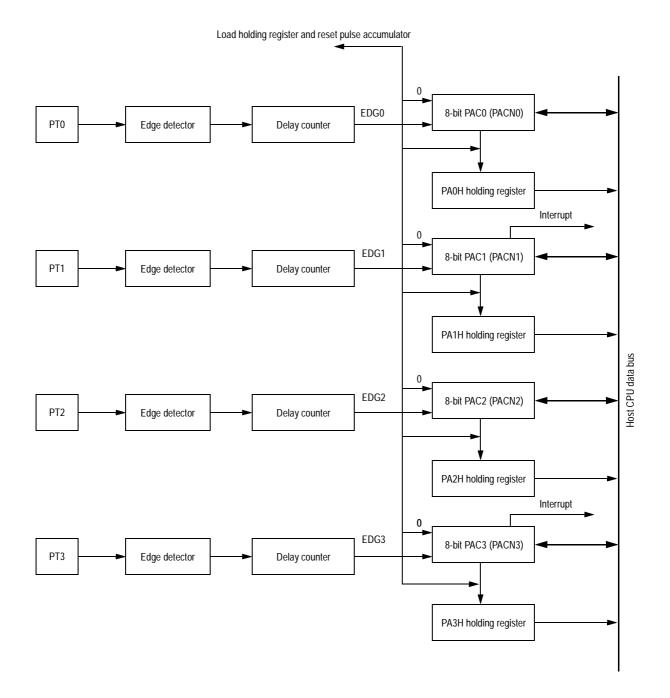
Figure 28 8-Bit Pulse Accumulators Block Diagram
