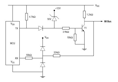
Figure 41 A typical MI Bus interface
